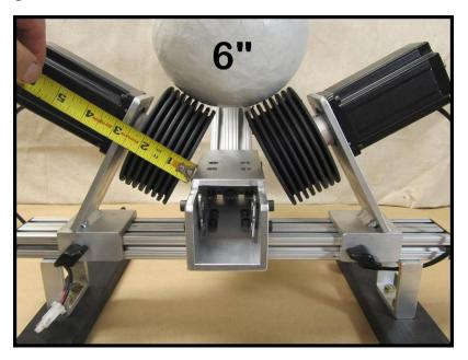
For 8" shells, increase the gaps to  $\frac{3}{4}$ ", and for 10" shells, to 1.25".
