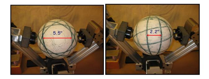
*Note*: After a test run, a damp rag can be used to clean the washable marker ink off of the dummy shell and the three Stinger rollers. A dry rag is used to then dry them before a subsequent test run.
