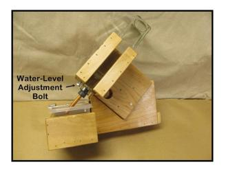
Water-Bottle and Bracket Installed, and Water-Level Adjustment Bolt
