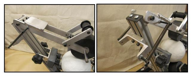
During taping, the tape-application wheel should ride centered slightly to the right of the shell's centerline:
