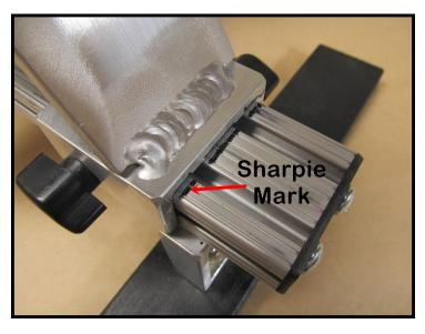
*Note*: Correct adjustment of this placement of the drive-wheels, per shell size, is important to the precise running of the individual taping programs. Remembering to make this adjustment will ensure consistent repeatability of the taping process.
