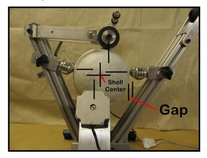
The position of the tape-application wheel is adjusted by loosening the bolts which attach the tape-application-arm to the left upright, raising or lowering that end of the arm, and retightening the bolts. Ensure that the arms which attach to the tape application wheel are parallel before their bolts are tightened.
