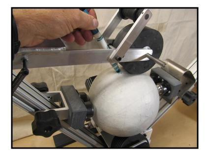
Clicking on "Start Full Run" starts to turn the shell in the machine. The marker will leave a mark that shows where the center of the tape would be applied with this program. I keep the marker centered on the face of the T.A. wheel.
