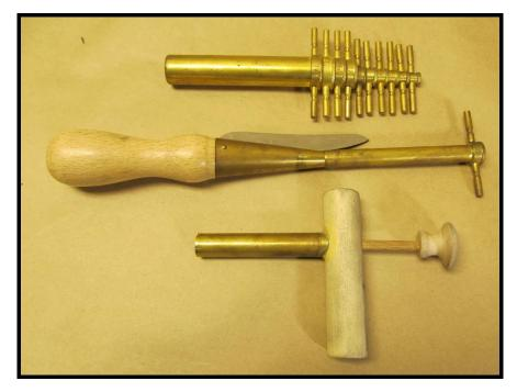
Once the magnet in a taped shell has been found using a stack of other magnets, the cork borer can be placed right over that stack, and twisted into the tape layers. A clean plug will be cut out of that taping, which is then pushed out of the borer with the plunger that comes with it, or is made to fit it.
