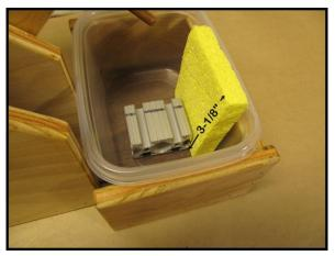
If more wetting area is desired, two or even three sponges can be installed, and held in place by reorienting the metal block.
