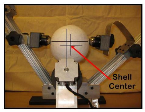
The shell should sit centered slightly to the right of the centerline of the drive wheels. The bearings should sit slightly above the shell's centerline.
