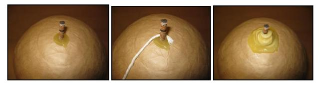
Once the glue is cooled, the fuse is ready to be cross-matched, and the shells can be lifted and leadered in the traditional ways.
