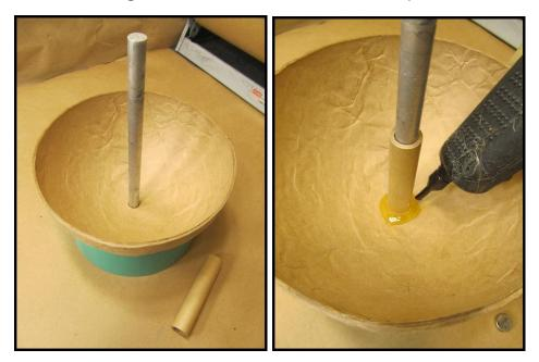
A <sup>1</sup>/<sub>2</sub>"-diameter magnet is pushed down through the passfire tube, and firmly into place in the casing's hole. Then the magnet is held in place with masking tape, securely stuck to it.
