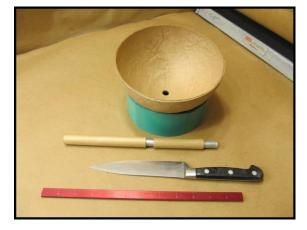
After a  $\frac{1}{2}$ " dowel is inserted into the casing's hole, the passfire tube is slid down over it, and hot-glued to the inside of the hemisphere.
