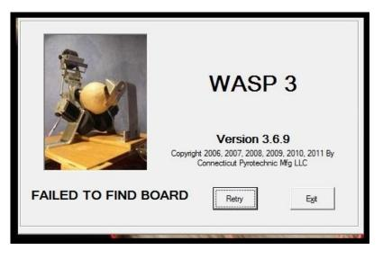
If that occurs, check all the cables, especially the USB cable from the controller to the computer, and the 110 volt power line to the power-supply, and click "Retry". If that doesn't solve the problem, click "Exit", check all the cables again, and open the program again, hopefully arriving at the "COM4: Model WASP3" window.
