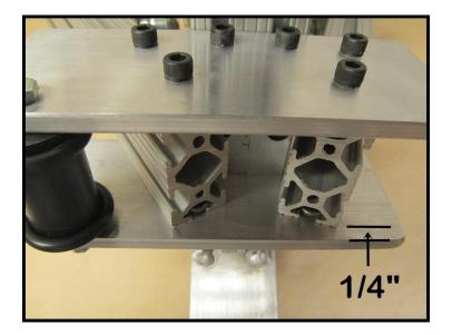
Make sure that the main-frame spine is square with the main frame, and centered on it, and that the bolts holding those parts together are nice and tight. Check all the bolts on the machine for tightness.
