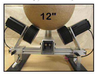
It can be handy to put Sharpie marks, perhaps color-coded for the different shell sizes, on the top of the crossmember at the appropriate locations so that the adjustments can be made quickly and evenly in the future.
