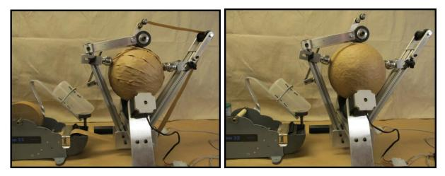
WASP Mini Taping an 8" Shell, and After Burnishing
