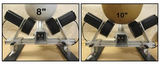
And, finally, for 12" shells, the gaps should be adjusted to 1.5".
