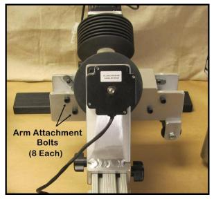
Use a 3/16" Allen wrench (hex key) to loosen those 8 bolts until their ends are just recessed in a little from the insides of their nuts. Line the nuts up so that their sides form a straight line.
