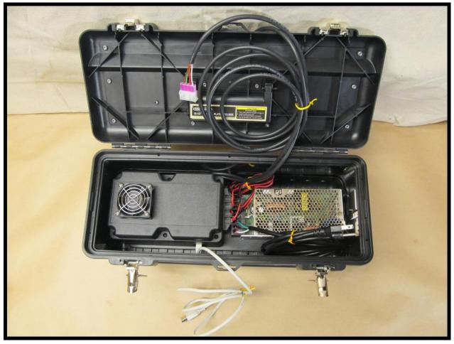
The components are simply held firmly to the bottom of the toolbox with heavy-duty two-sticky-sided tape. I like to refer to this as my "WASP-in-abox". I've installed a ground wire from the electronics "ground" to the toolbox's metal sides, and have also installed wire-straps to strain-relieve the wires as they exit the toolbox.
