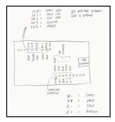
If you open the controller box, you'll see the circuit board that the schematic refers to:
