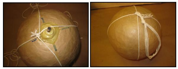
When the shell is lifted, the strings will pull away from the shell down to the equator, so don't glue the strings to the shell above the equator.
