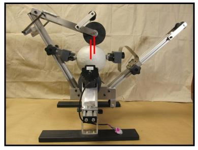
If the bolts that attach the tape-application arm to the left upright are loosened, and the left end of the TA arm is moved downward, the TA wheel will move to the right, and vice versa. That is how the position of the TA wheel is adjusted to sit correctly atop a shell. After the correct position is attained, verify that the TA arm is aligned with the two uprights, and retighten the bolts.
