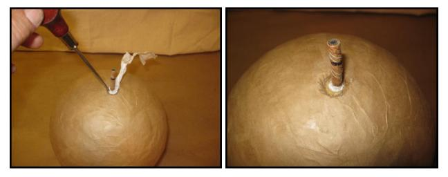
Now, the purpose of the two methods described below is to seal that hole in the shell's casing around the fuse. Making a solid, strong seal which will prevent lift gasses from entering the shell, and which will shed fire away from that area, is paramount to getting the shell out of the mortar safely.
