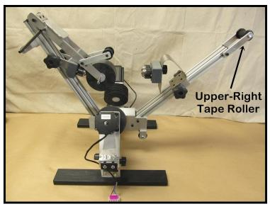
For the tape to run evenly, and centered, over that upper-right tape roller, it is important that it be straight and level. If, during WASPing a shell, the tape does not stay centered on that roller, the bolts can be loosened and the alignment of that roller can be adjusted.
