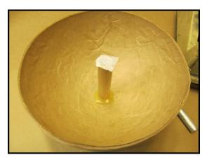
Now, the shell casing is ready for standard shell assembly. After this assembly, the seam between the shell hemispheres needs to be completely sealed with masking tape. At no time should a shell with any openings in its casing be put on a powered-up WASP machine for taping.
