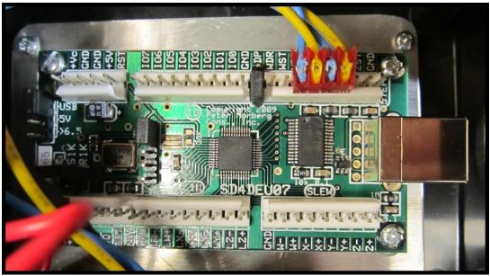
The lower right strip of terminals is labeled "Slew". Per the schematic, if a connection is made between the "GND" (Ground) pin on that strip, and the pin marked "W-", the machine will "start". A connection between GND and W+ will cause the machine to pause, X+ to Burnish, and X- to Stop.
