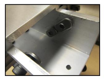
Now carefully slide the left and right arms into place, so that those nuts slide up into the side-channels of the arms. This can be a bit tricky, but you'll succeed with a bit of patience. Press the arms all the way down until they bottom out on the bottom of the spine, and tighten the bolts.
