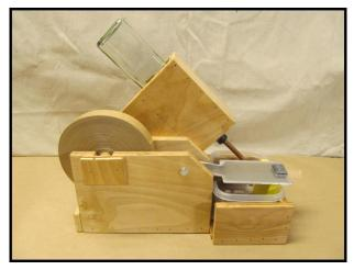
To fill the wetting station with water, fill the plastic tub about 2/3 full of water, and then fill the water bottle, ensuring that the rubber stopper is securely in place afterward. While holding a finger on the end of the bottle's copper water spout, slide the water bottle down into its holder. Now allow water from the bottle to fill the tub up to the end of the copper spout.
