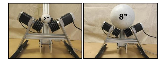
As shown in the next photo, the left and right ball bearings should be adjusted so that they sit just above the shell's centerline. The shell should sit just to the right of the motors' center, and the tape-application wheel should sit just to the right of the shell's center.
