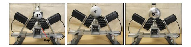
For 6" shells, increase those gaps to 3/8". You can see how that causes the shell to ride right in the middle of the drive rollers.
