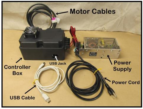
The power supply is connected to the controller with 2 pairs of red and black wires, and it also has a power cord to plug into a standard power outlet. The red and black wires may be shortened as desired, and their connectors reoriented as necessary.
