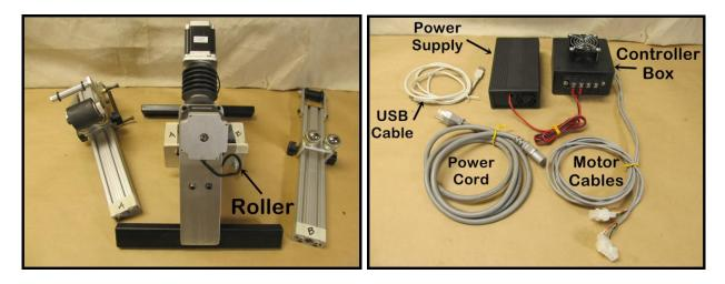
Notice that the roller on the bottom of the drive-wheel-frame is on the right, and that the arms are labeled "A" and "B" to match with the same labels on that drive-wheel-frame.
