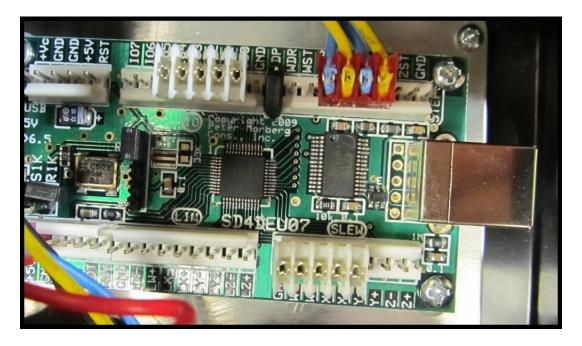
In the simple example of my two-switch box, the black wire is connected to GND on the SLEW strip, the Green wire (Start) is connected to the W-terminal, and the Red wire (Pause) is connected to the W+ terminal.
