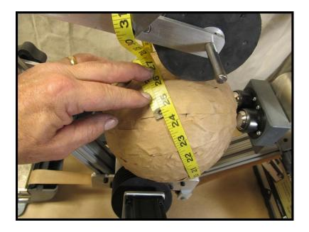
Once the taping program terminates, the tape is torn at the top of the shell, and the "Burnish" run is initiated. The tape really gets packed down into a solid, single layer in that process.
